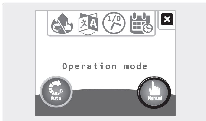
Fig. 3.21 Touch control panel – Manual operating mode
