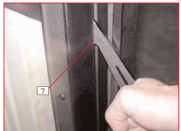
Figure 4: closed hatch blocked (rotate the pallet by 90°)
